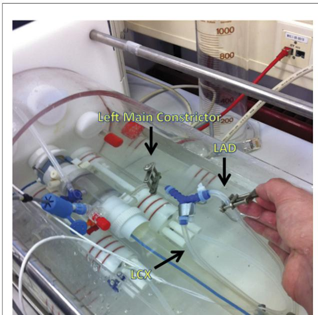
**Figure 1. In Vitro Model of the Coronary Circulation**
